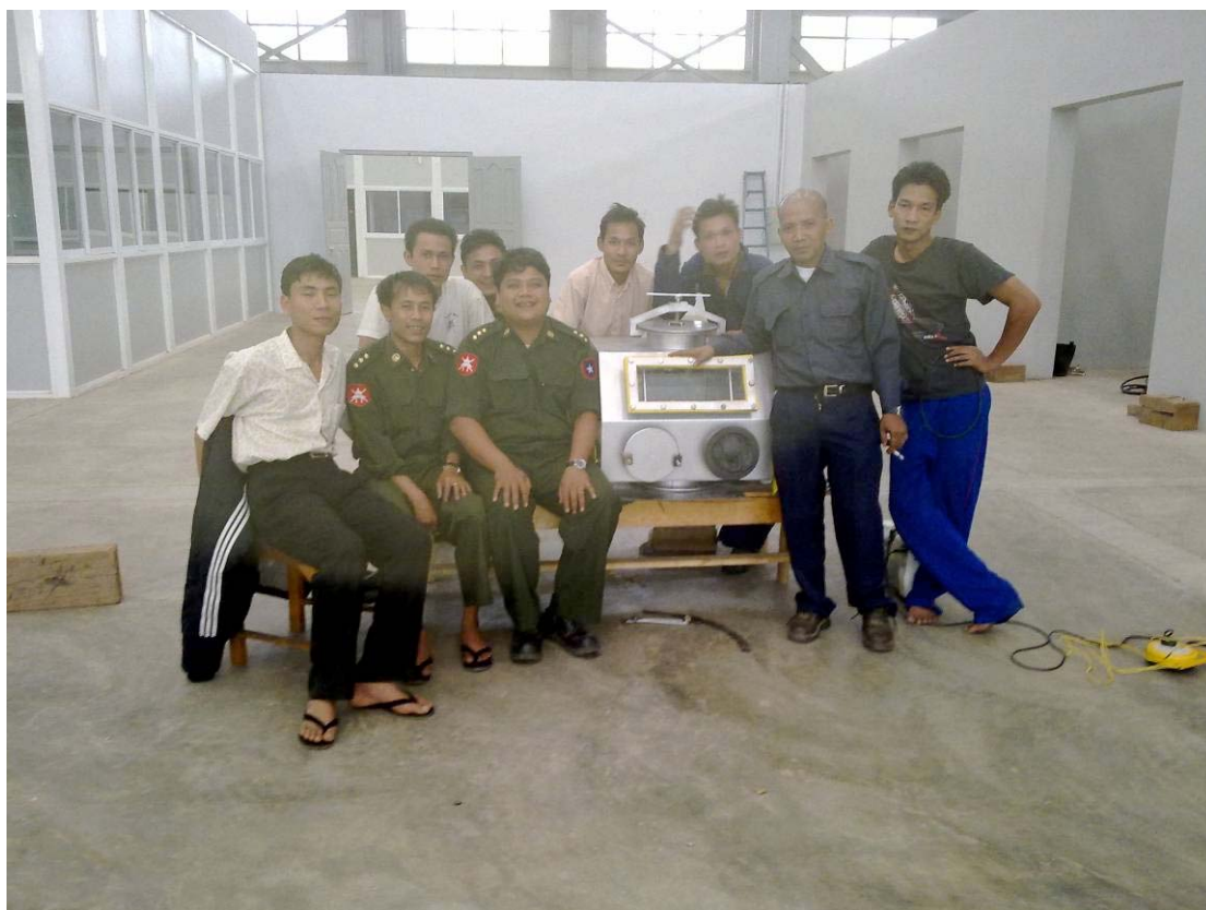
Figure 14. Inert Atmosphere glove box. Vacuum pump is behind the man on the right.
