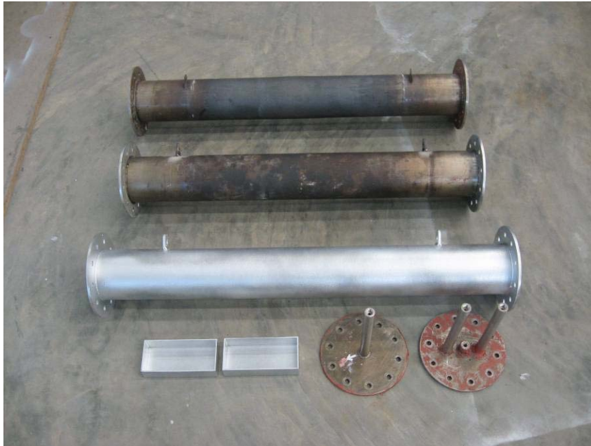
Figure 18. Two used tube furnaces and one new one
