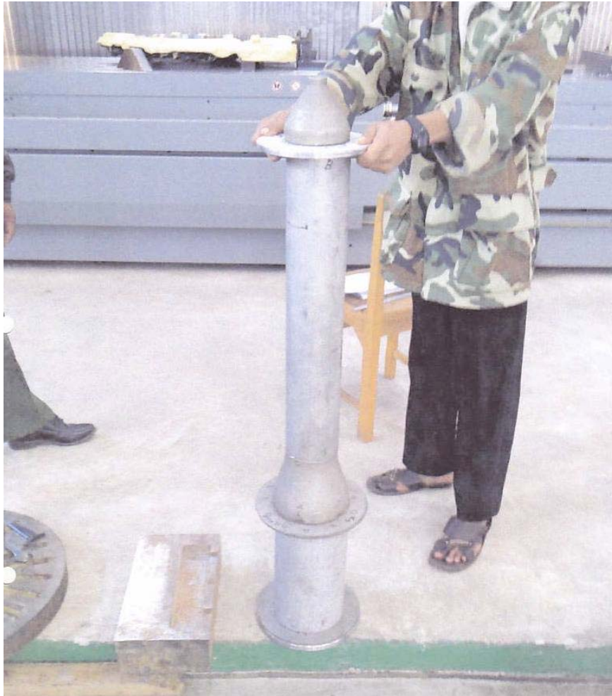
Figure 17. Presumed Inconel tube with the section surrounded by the furnace in the previous figures
