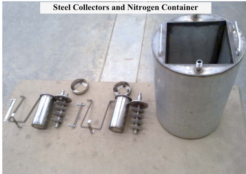
Figure 19. Possible cold trap assembly for collecting \text{UF}_6 gas
