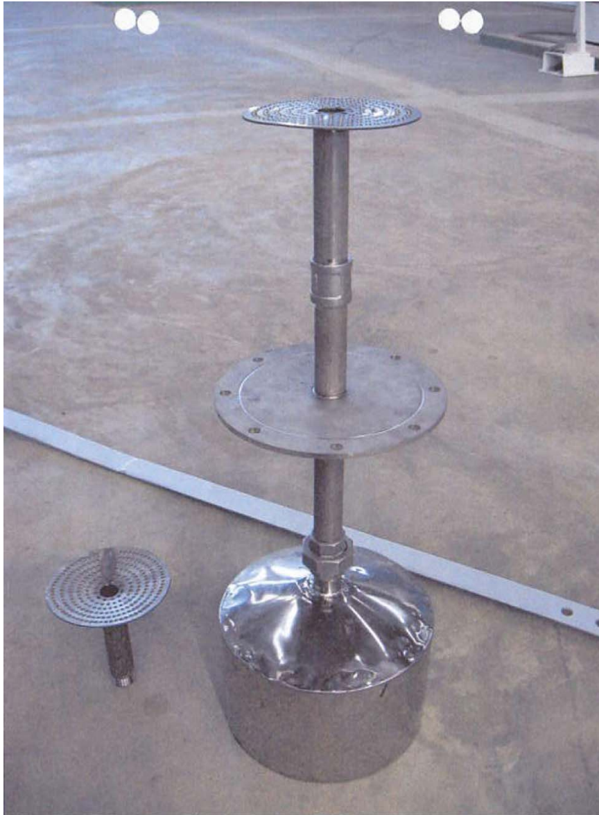
Figure 16. Internal components of the “Fluoride Bed Reactor”
