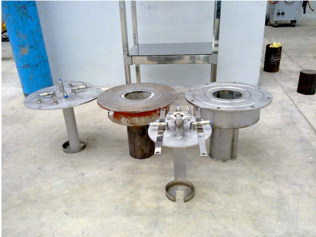
Figure 13. Two bomb reactors, one used and one new
